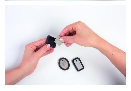
The **temperature** and **humidity** are decisive for the drying time. However, it is advisable to remove the trailer from the mould the **next day**. The upper side, i.e. the later back side, can be dried with a fine **Sandpaper** straightening and smoothing.
